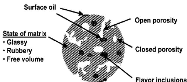
**Figure 1. Structural defects in glassy encapsulation matrices. (Ubbink et al, 2003)**
