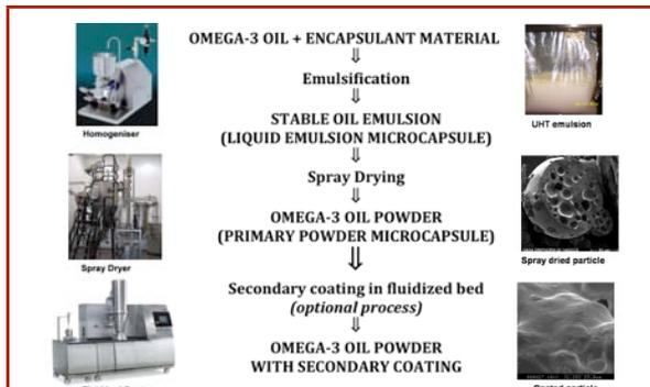
Figure 3: Standard microencapsulation process using MicroMAX® technology involving the formation of stable emulsion, which can be spray dried into powder and optionally be further coated with another layer of encapsulant material to tailor the release characteristics of the final microcapsule.
