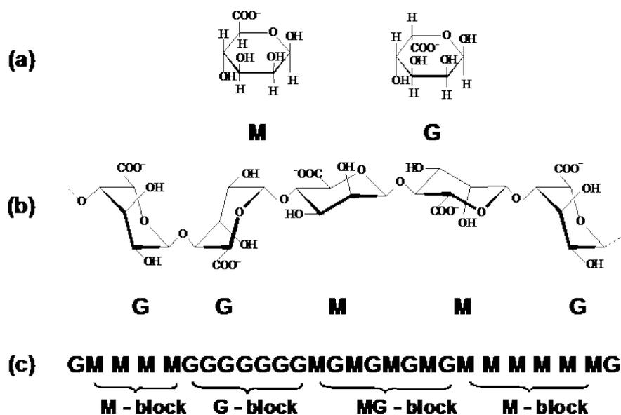
Figure 2. Structure of alginate.  $\beta$ -D-mannuronic acid (M) and D-L-guluronic acid (G). Haworth formulas (a), ring conformation in the alginate chain (M: 4C1 and G: 1C4) [6](b), and the alginate chain sequence (c).
