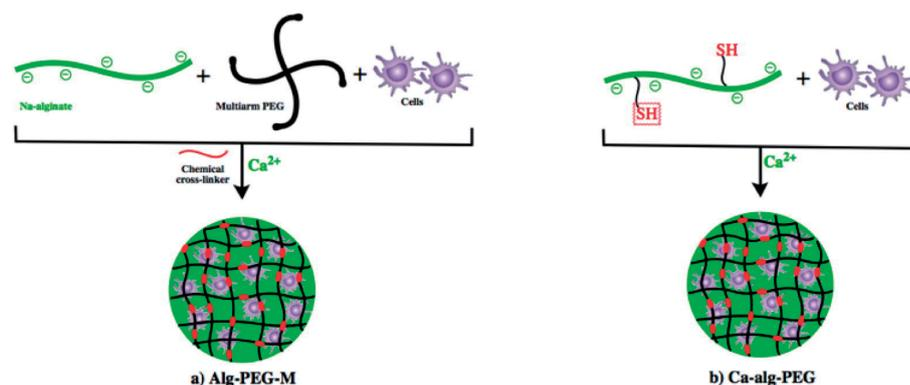
Figure 3: Two strategies to produce hydrogel microspheres by a one-step technology
