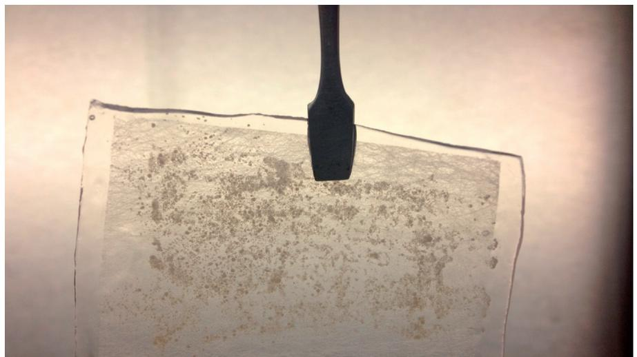
Fig. 1 Islet Sheet made from piglet islets, 3% alginate and polyester scrim
