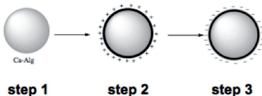
Figure 2: Multi-step technology, consisting of gel formatting, coating with polycation and polyanion, as well as washing steps, to adapt the physical properties for cell transplantation
