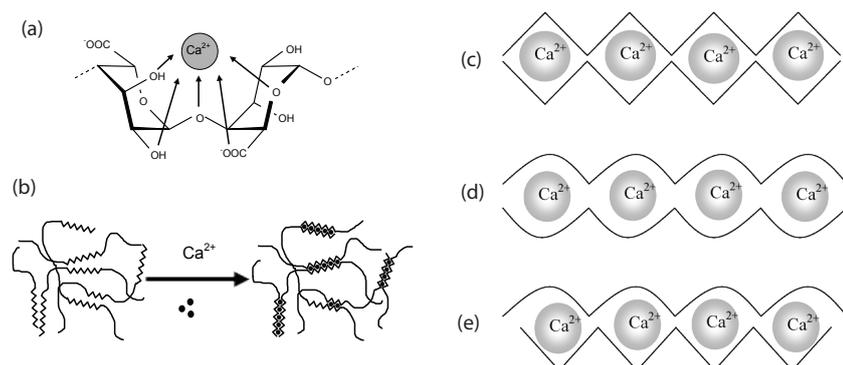
Figure 3. Crosslinking alginate polymers by calcium ions. Probably Ca-binding site in a GG-sequence [a] and ionic cross-linking of two homopolymeric blocks of G-residues by the egg-box model [b] [19]. [c] GG/GG junctions, [d] MG/MG junctions [e] GG/MG junctions [17].
