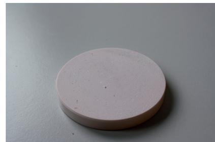
Figure 2. Fabricated sample composed of Ca-alginate microspheres incorporated into W19 commercially available low loss epoxy material.
