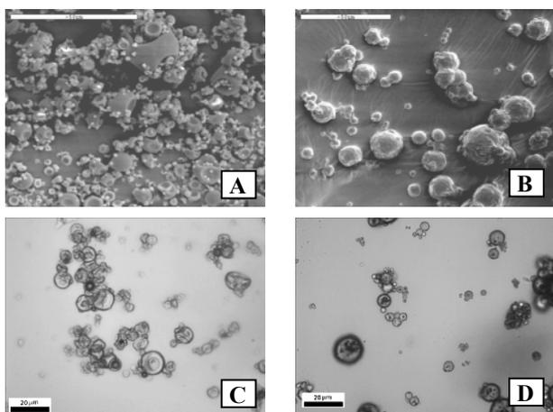
**Figure 2: Morphology of microparticles. Spray Drying: A – SEM, (700X, bar = 50  $\mu\text{m}$ ); C – MO (200X, bar = 20  $\mu\text{m}$ ). Spray Chilling: B – SEM, (500X, bar = 50  $\mu\text{m}$ ); D – MO (200X, bar = 20  $\mu\text{m}$ ).**
