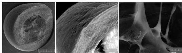
**Figure 5. Structure of capsule after preparation.**
