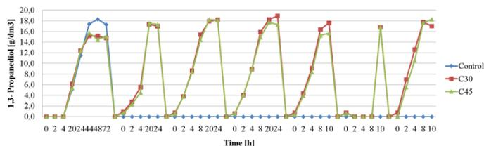
**Figure 1. Concentration of 1,3-propanediol during the bioconversion process by encapsulated *Citrobacter freundii*.**
