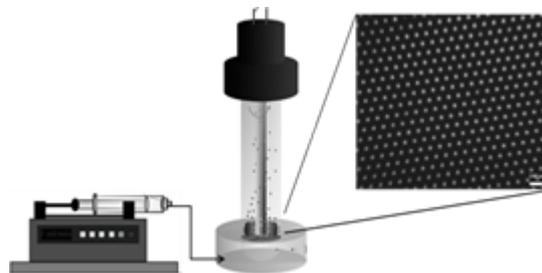
**Figure 1: Schematic of the Stirred Cell equipped with a hydrophobic 20 µm pores nickel membrane**
