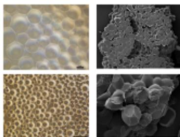
Figure 3. Microscope photographs of particles and SEM analysis confirming particles with solid core
