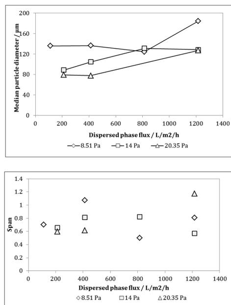
Figure 2. Effect of dispersed phase flux and shear stress on the median particle diameter
