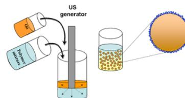
Fig. 1. The schematic representation of the microcontainer formation.
