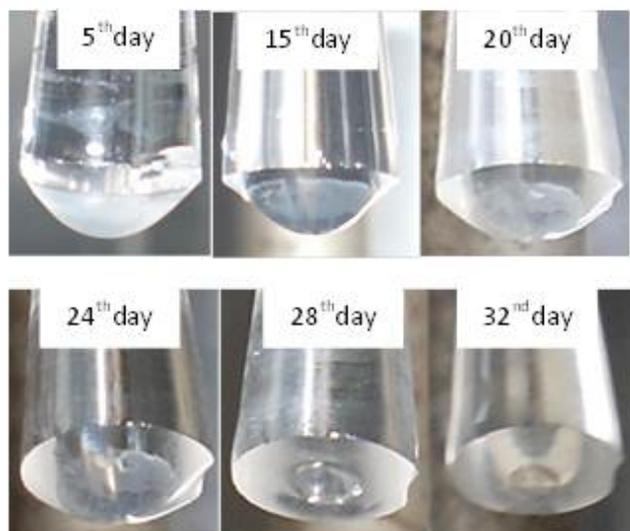
**Figure 2: The silica gel lens with entrapped *Pseudomonas putida* TVA8**
