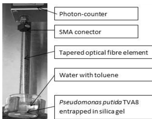
Figure 1: The tapered optical fiber element connected with photon counter
