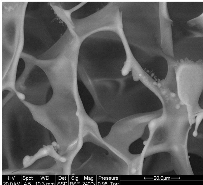
**Figure 2: SEM of freeze-dried gel Amylopectin/Concanavalin A/salts.**
