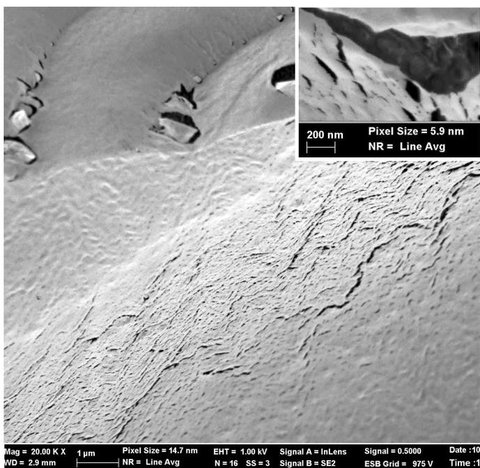
**Figure 3: HR-Cryo-SEM of vitrified and fractured gel Amylopectin/Concanavalin A/salts at the magnification 20 000×. In the insert the magnification is 50 000×.**
