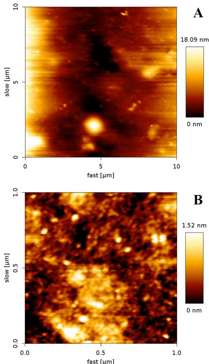
**Figure 1: AFM of dried 8% amylopectin gel, crosslinked with Concanavalin A in the presence of salts, imaged in the intermittent contact mode in air.**
