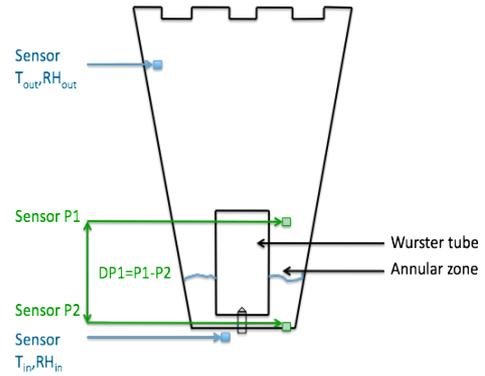
**Figure 1: Measures for the automatic control process**
