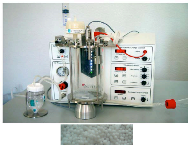
Fig. 2. Encapsulator for making uniform gel beads.
