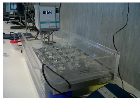
Figure 1 : Experimental set-up with Franz-diffusion cell
