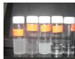
Figure 1: Nanogels at room temperature. From left to right: PNIPAM, PNIPAM-MA, PNIPAM-AAc, PEG.PNIPAM, PEG.PNIPAM-AAc
