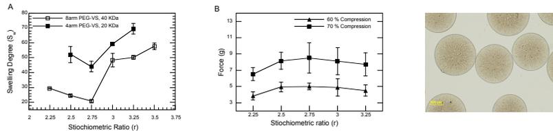
**Fig.2.** Left: Swelling degree (A) and Mechanical resistance (B) as a function of  $r$ . Right: Alg-PEG beads hydrogel formed following the described method.
