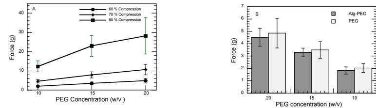
**Fig.4.** Mechanical resistance as a function of PEG concentration (A), and the effect of alg layer on mechanical stability at 60 % (B).
