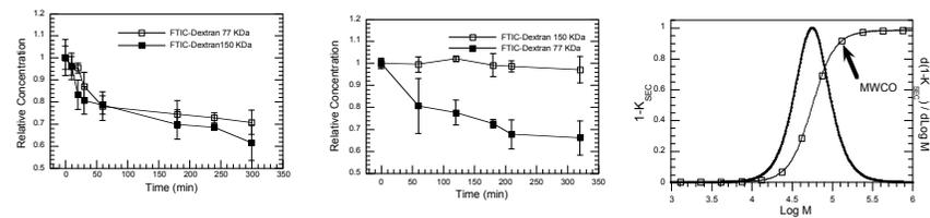
**Fig.3.** Diffusion of labeled dextran into alg-PEG hydrogel. Left: Hydrogel formed using PEG 40 KDa, middle: hydrogel formed using PEG 10 KDa. Right: ISC curve for hydrogel formed using PEG 10 KDa.
