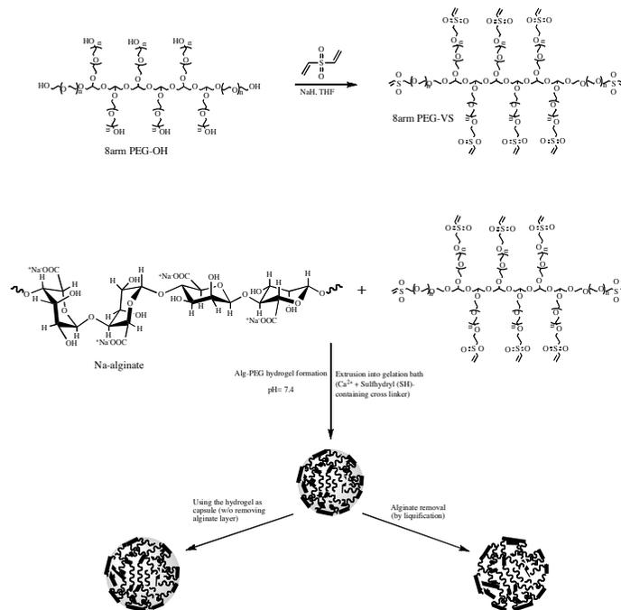
Fig.1. Schematic representation of the followed approach for alg-PEG hydrogel formation.
