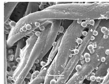
Figure 6: SEM of Triclosan microcapsules on a woven cotton textile after standardised washing at 40°C
