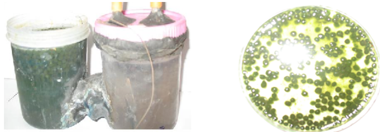
Figure 1. Entrapped algal bead in cathode (left hand side) Figure 2. Entrapped algal beads
