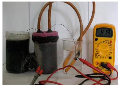
Figure 3. Experimental setup of microbial fuel cell
