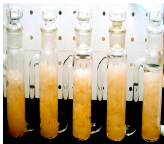
Fig. 1 Setting of reactor for wastewater treatment using resting cells of Nocardia globerula entrapped in agar gel discs.
