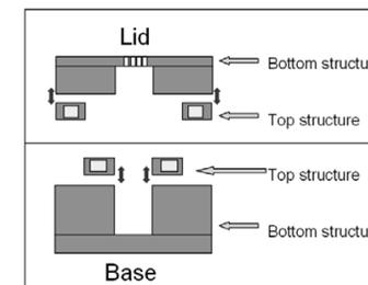
**Figure 2:** The based and lid each contained two discrete components that were bonded together using a nanoimprinter.
