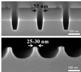
**Figure 3:** The nanoimprint mold (top panel) was cyclically oxidized and etched to reduce the feature size (bottom panel) until the desired 15 nm thickness was achieved.
