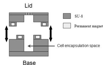
**Figure 1 :** The SU-8 base and the nanoporous lid of the microcontainers have permanent magnets embedded in them to aid in assembly and to close the device once it is filled with cells.
