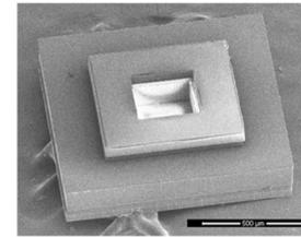
**Figure 5:** The two discrete components of the base were bonded together using a nanoimprinter. The resulting structure, seen above, was well-aligned so as to accommodate cells in its hollow space, and eventually the nanoporous lid. The lid was similarly bonded.
