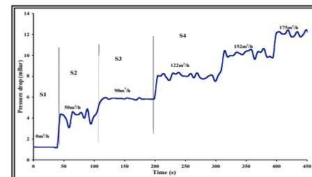
**Figure 3 : Reactor pressure drop in Wurster reactor**
