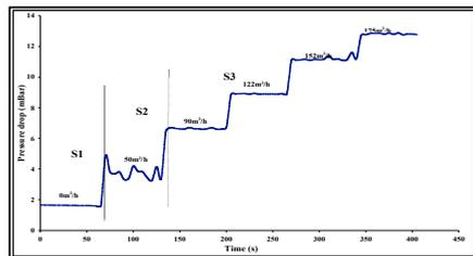
Figure 3 : Reactor pressure drop in spouted bed
