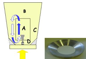
**Figure 2 : spouted bed reactor and insert**
