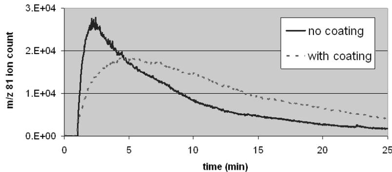
Figure 3: Absolute flavour release from granulated spray-dried lemon flavour with or without a water-insoluble coating at 80°C and equal flavour load as measured by PTR-MS.
