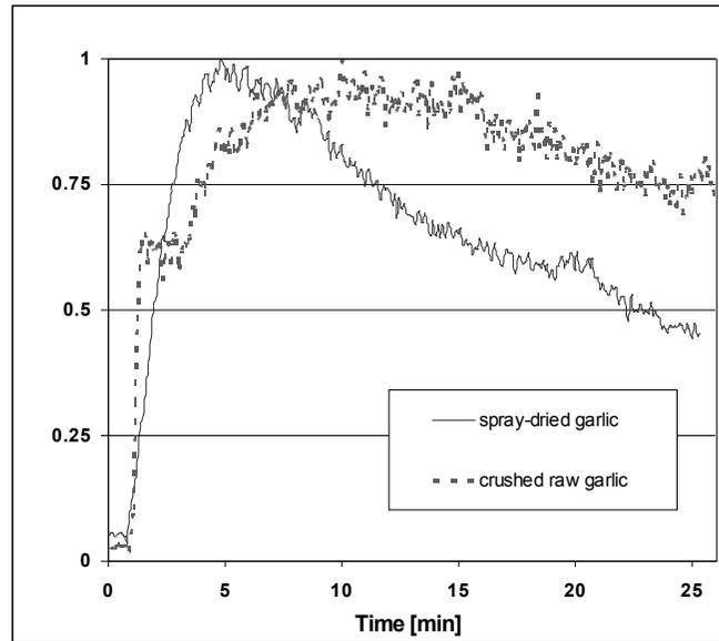
Figure 2: Garlic release from spray-dried encapsulates or crushed raw garlic in water at 80°C as measured by PTR-MS. The maximal response was set at 1.
