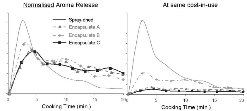
Figure 4: Flavour release from spray-dried and commercial encapsulates in water at 80°C as measured by PTR-MS. The release curves were normalized as such that the area under the curve was the same for each sample. The left picture shows the results at equal flavour load, and the right picture shows the results at equal costs. These data were kindly provided by our colleagues S. Coić and D. Taal.
