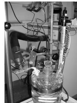
Figure 1: Set up for controlled aroma release measurement of encapsulates by PTR-MS.
