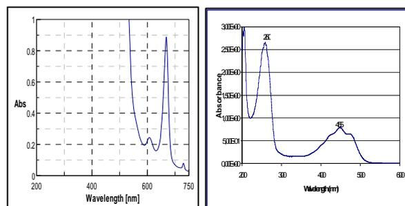
Fig. 4. UV-Vis spectra of HDF: phenolics ( $\lambda_{\max}$ =280 nm), carotenoids ( $\lambda_{\max}$ =450 nm) and chlorophylls ( $\lambda_{\max}$ =610 and 660 nm) identified.
