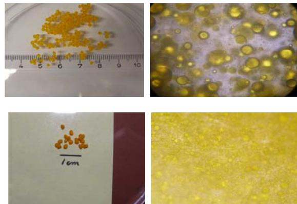
Fig.2.General aspect and dimensions of microcapsules SBO-C and LDF (up) and HDF-C1 and HDF-C2 (down)
