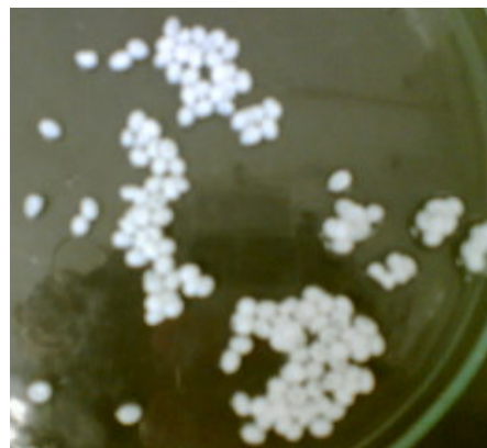
Fig. 4: PVAL particles of immobilized cutinase
