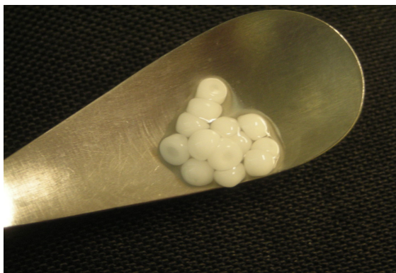
Figure 1: Typical shape of PVA capsules obtained following extrusion polyethers. The capsules depicted were obtained in in PEG 600.
