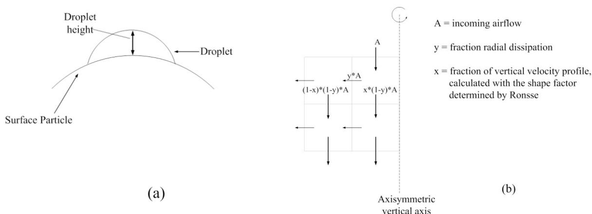
**Figure 3. (a) Droplet on particle, (b) Modelled airflow pattern**
