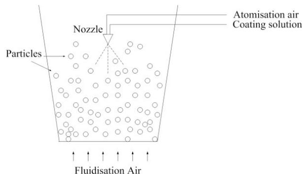
Figure 1. Fluidised bed coating reactor
