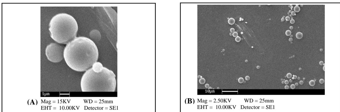
**Figure 3. Scanning electronic photomicrographs of Cubebin loaded PLGA microparticles: (A) isolated magnified particle and (B) panoramic view of Cubebin loaded PLGA microparticles.**
