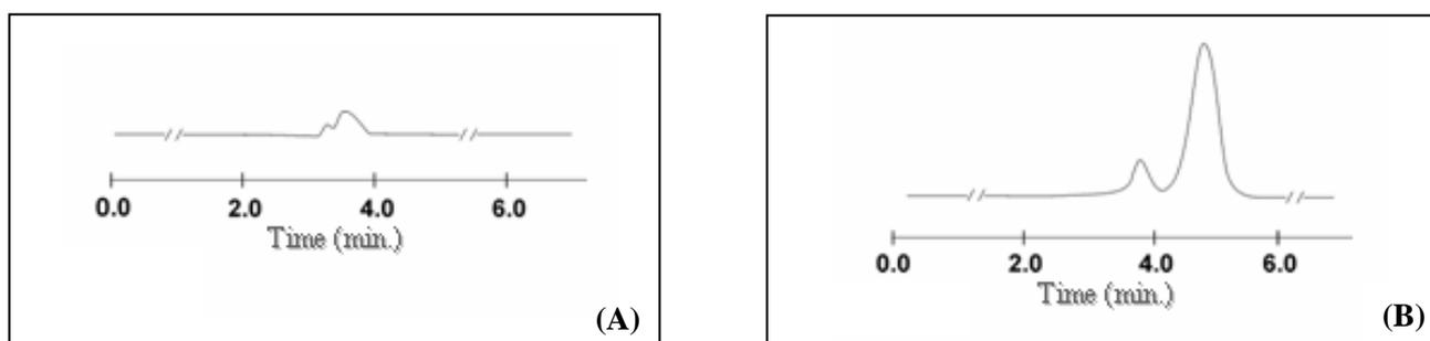
**Figure 4. Chromatograms of inert PLGA microparticles sample (A), Cubebin microparticles sample about 6 $\mu\text{g}$  of Cubebin/mL (B). Retention time of Cubebin was 5.0min. Chromatographic conditions:  $\text{C}_{18}$  reversed-phase column shim-pack (250x4mm, particles of 5 $\mu\text{m}$ ) and a  $\text{C}_{18}$  pre-column shim-pack (4x4mm, particles of 5 $\mu\text{m}$ ), mobile phase acetonitrile: water 60:40 (v/v), at flow rate of 1.0mL/min, detection at 285nm.**
