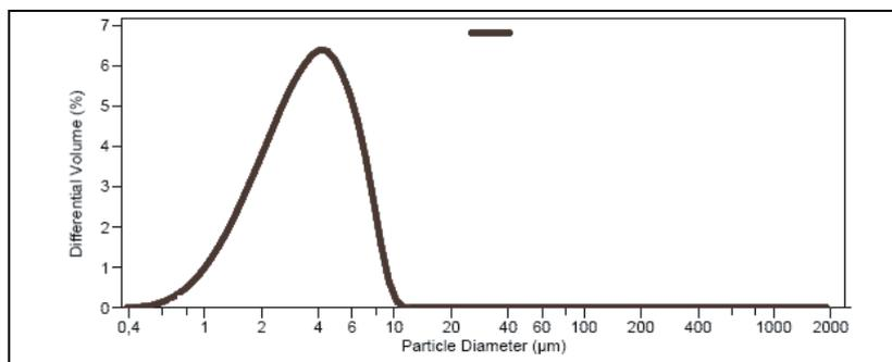
**Figure 2. Size distribution of Cubebin loaded PLGA microparticles.**
