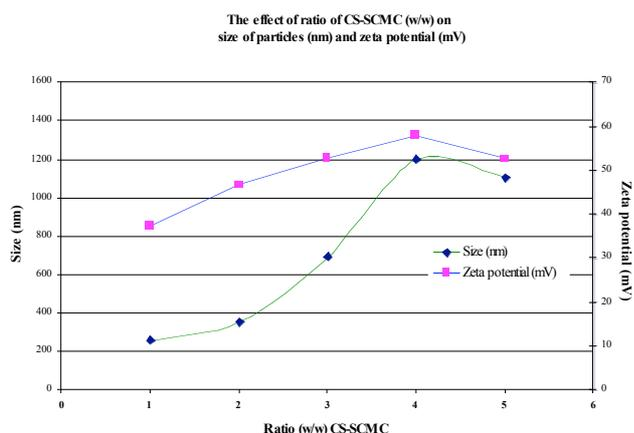
**Figure 1. The effect of ratio of mixing of CS and SCMC on size, size distribution and surface-charge of the CS-SCMC nanoparticles**
