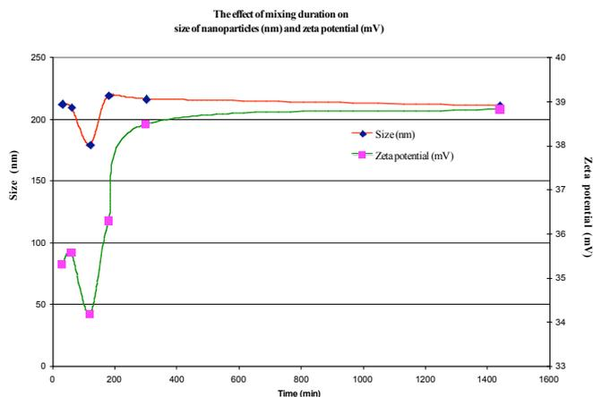
**Figure 2. Effect of mixing duration of CS and SCMC on size, size distribution and surface-charge of the CS-SCMC nanoparticles**
