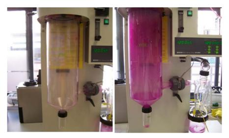
Figure 1. Powder stickiness on dryer chamber during spray drying of 10% (v/v) *O. stricta* juice (left) and 80% (v/v) *O. stricta* juice (right). Ratio DGS/juice is 1.66.
