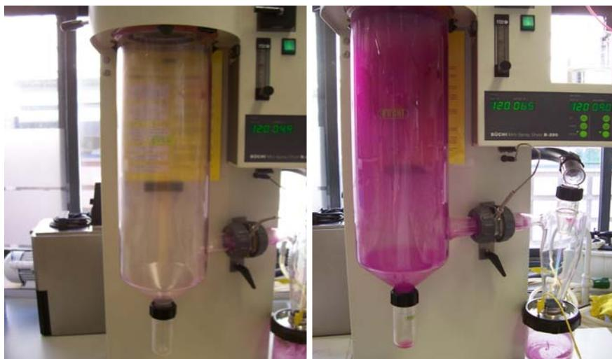
**Figure 1. Powder stickiness on dryer chamber during spray drying of 10% (v/v) *O. stricta* juice (left) and 80% (v/v) *O. stricta* juice (right). Ratio DGS/juice is 1.66.**
