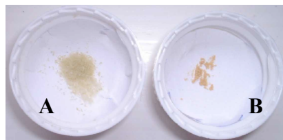
Fig. 4 The appearance of CAE entrapped in nanoparticles (A) and CAE intact (B)
