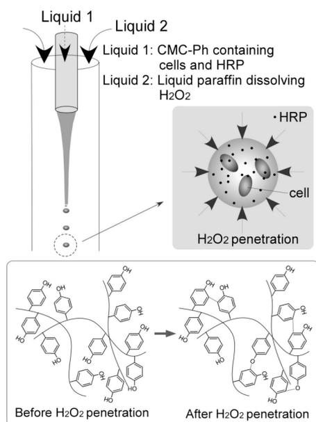
**Figure 1:** Schematic illustration of breakup of cell enclosing droplets via jetting and gelation via HRP reaction
