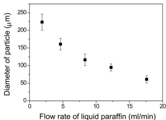
**Figure 2:** CMC-Ph particle diameter as a function of the velocity of liquid paraffin.
