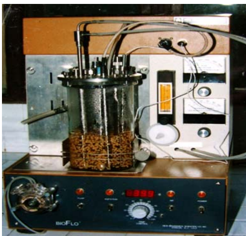
Fig. 1 Batch synthesis of acrylic acid using resting cells of Rhodococcus rhodochrous entrapped in polyacrylamide gel discs.
