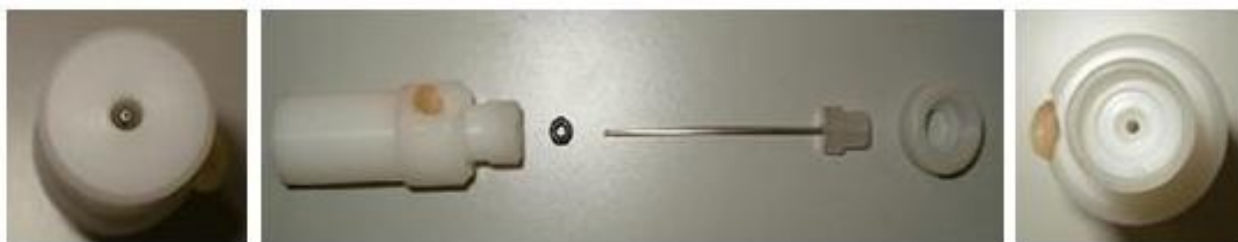
Fig. 1. The flow focusing device LB-EXT/1 used for the preparation of solid lipid microparticles
