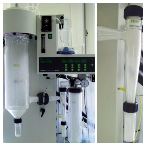
Figure 1: Mini Spray Dryer B-290 with High Performance Cyclone during spray drying of biodegradable polymers.
