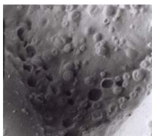
Fig. 3: Textile impregnated with essential oil microcapsules
