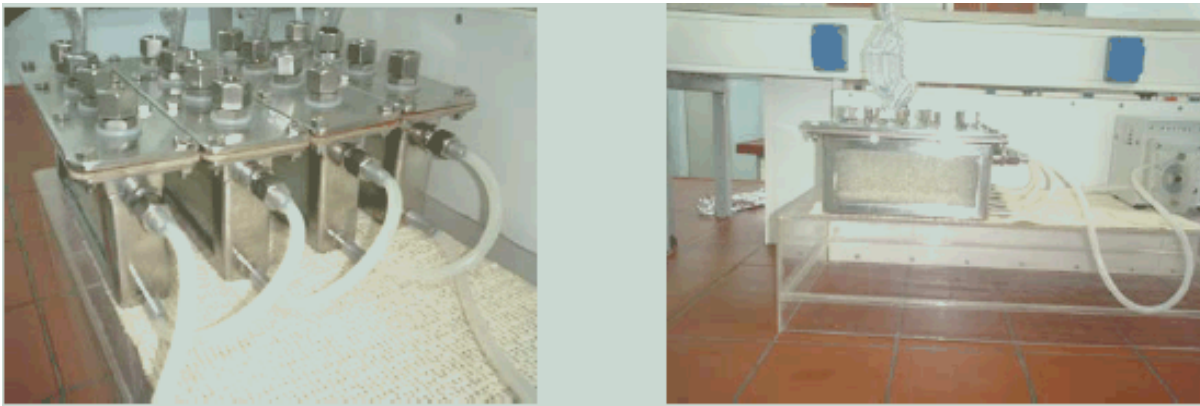
Photos 1. Photos of the actual MicroFermentation Cassettes, .1 st photo (connections of four cassettes in series), 2 nd photo (microencapsulated yeast cells in the cassettes).
