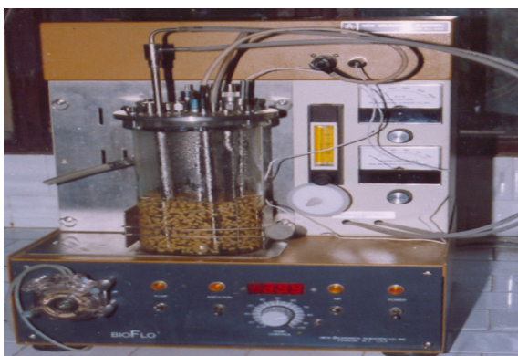
Fig. 1 Setting of batch synthesis of AHA using resting cells of Nocardia globerula entrapped in alginate gel beads.
