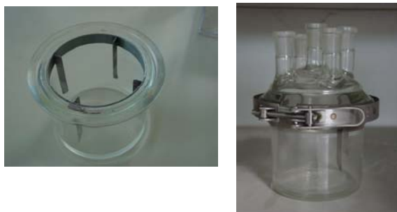
Figure 2: Beaker with baffles (left); Beaker fixed with the cover (right)
