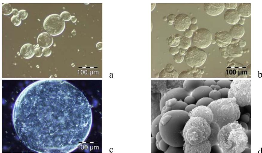
**Figure 1. (a-c) Microphotographs of PGA-HSA coated microspheres. (a) small MS, gelation with CaCl<sub>2</sub> 20 %; (b) small MS, gelation with CaCl<sub>2</sub> 5 %; (c) large MS, gelation with CaCl<sub>2</sub> 20 %, (d) SEM observation of THP-1 cells in contact with the MS (magnification x3500).**
