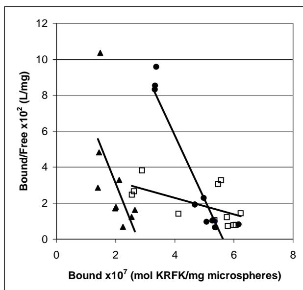
**Figure 3. Scatchard plots of KRFK interactions with the microspheres.** (●) small MS, gelation with CaCl<sub>2</sub> 20 %; (□) small MS, gelation with CaCl<sub>2</sub> 5 %; (▲) large MS, gelation with CaCl<sub>2</sub> 20 %.
